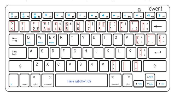
Keys Android - USE "FN" KEY + "W" FOR OPERATING IN ANDROID
